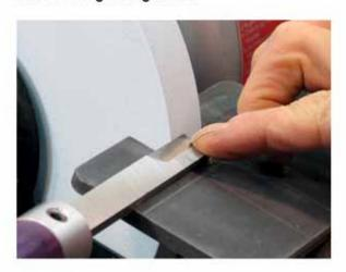
It is important that the end cutting edge remains perpendicular to the side of the tool and the side cutting edge remains parallel to the other side. I have made some reference marks on the grinder platform to help my eye line the edges up.
